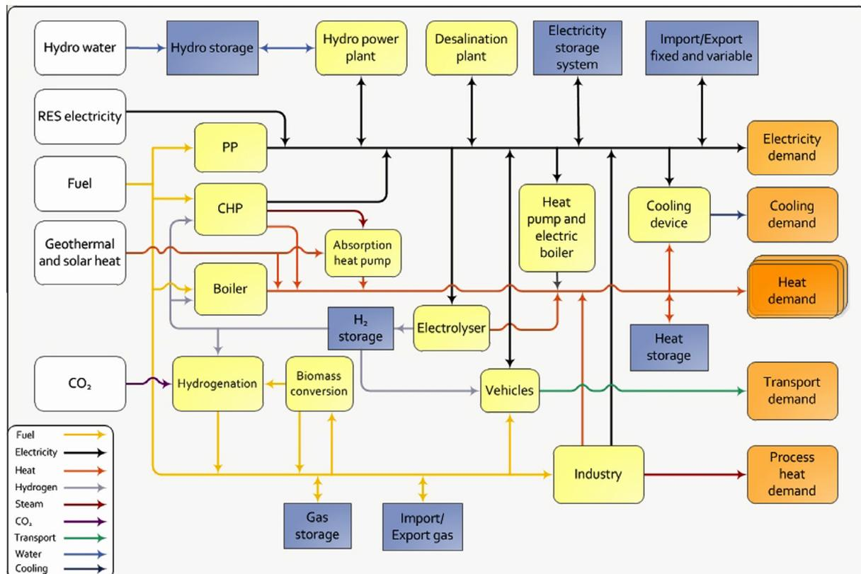
Fig. 1. The EnergyPLAN model in version 11.4 [40].
