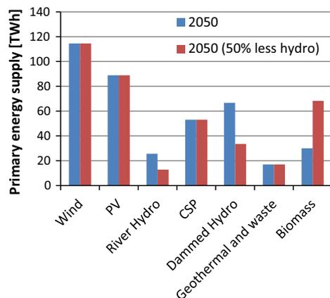
**Fig. 5.** Difference in electricity generation during sensitivity analysis.
